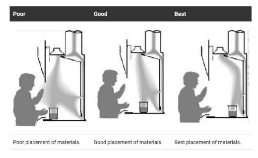
Work as close to the center of the hood as possible and at least 6 inches back from the sash opening. A vortex forms in front of your body that can cause contaminants to flow out of the hood.
