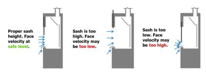
Variable Air Volume (VAV) hoods vary the air flow to maintain a constant face velocity regardless of the sash height.
