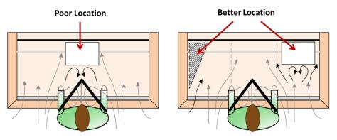
• Do not block slots. If large equipment must be placed in the hood, put it on blocks to raise it approximately 2 inches above the surface so that air may pass beneath it. Place large or bulky equipment near the rear of the fume hood. Large items near the face of the hood may cause excessive air turbulence and variations in face velocity.
