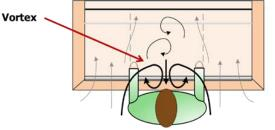
• Large equipment can create vortexes and can block the slots used to exhaust the air, which can cause contaminants to flow out of the hood. Position large equipment to the side when possible and place equipment on blocks to prevent it from blocking the back slot.
